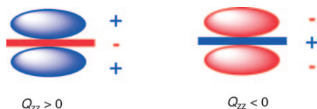
Figure 2. Schematic side view of \pi -acidic (left) and \pi -basic (right) aromatic rings (solid lines) between their electron-poor (blue) and electron-rich (red) \pi -clouds, with indication of the negative and positive axial quadrupole moments Q_{zz} that are used to quantify \pi -basicity and \pi -acidity, respectively.
